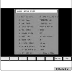
Use [1] . Then the screen like 'Fig. 3.2.1 Embroidery Machine Specifications Setting' appears where the setting of each item is possible. When the setting is completed for all items, press [7] NEXT . <Fig. 3.2.0-2> appears to check the set specifications.
