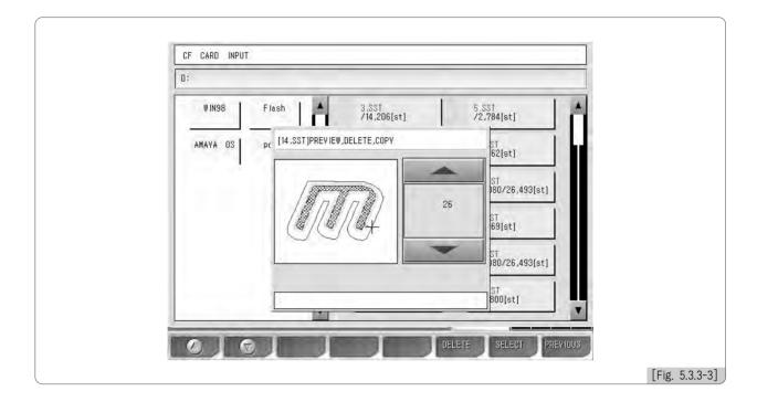
In the USB memory, the preview function can be directly performed. Copy and Delete buttons also exist at the bottom. Preview, Delete, and Copy functions can be used in the same way as explained in "5.3.1 FDD Input".
