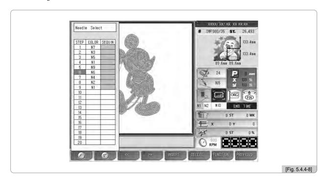
**5** Use the direction buttons and move the cursor to "4" under #7 needle bar. As in <Fig. 5.4.4-9>, the cursor will move to the "4" position.
