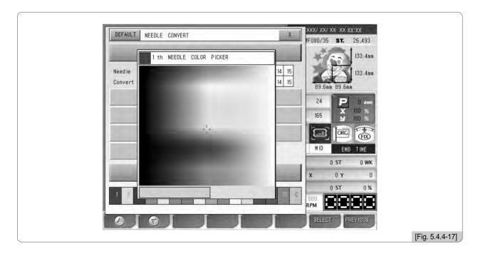
On the color change window in <Fig. 5.4.4-17>, use the frame speed key to adjust the cursor move speed.
