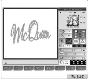
If there are no designs called as in <Fig. 5.2-1>, several function buttons cannot be used. The buttons whose letters are pale cannot be used until the designs are called later.
