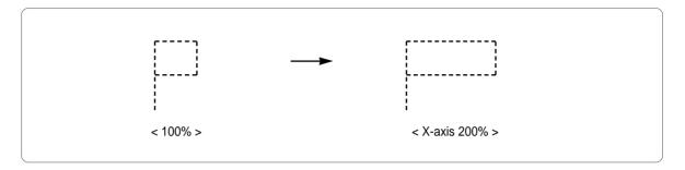
The default is 100%, and the value can be adjusted from 50% to 200% by the unit of 1% .
