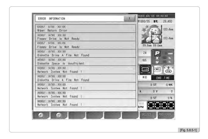
SWF system can save up to 10 error messages for the errors which occurred during operation. This function displays the details of the errors saved in the memory. By reading the details of errors, the causes of problems can be easily found.
