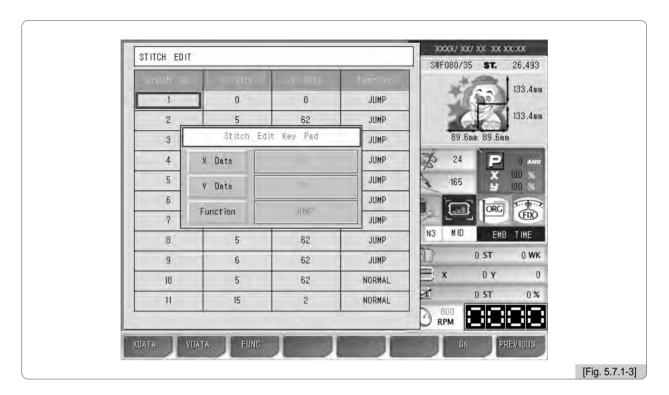
Press F3 FUNC, and as in <Fig. 5.7.1-4>, the menu for setting function codes is enabled.
