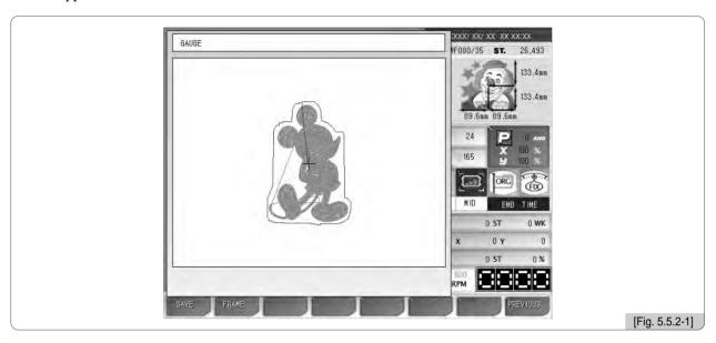
② Press FI SAVE in <Fig. 5.5.2-1>, and as in <Fig. 5.5.2-2>, the menu for design saving will appear. Select the room to save the design and press F7 COPY, and the design will be saved in the memory. To cancel the saving, press F8 PREVIOUS.
