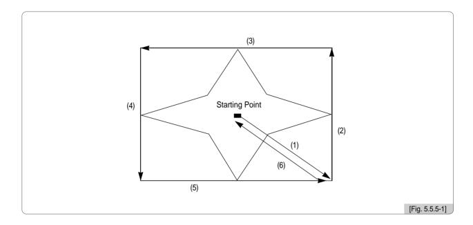
② The arrow marks in <Fig. 5.5.5-1> show the feed route of the frame. While the frame moves fast between the maximum X,Y range and the minimum X,Y range, the function checks whether the design goes beyond the frame limits. If so, the frame operation will be stopped, and the message "Frame Limit Error" will appear on the screen.
