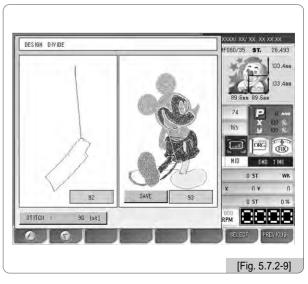
4 Press [1] , [2] to select the room numbers for saving and press [7] SELECT. Design saving is made in Room 92 and 93.
