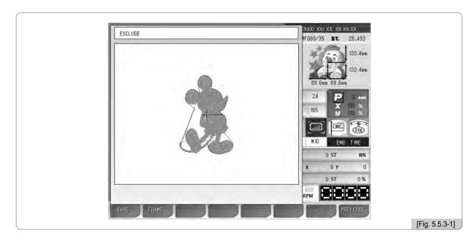
② Press F1 SAVE in <Fig. 5.5.3-1>, and then the menu for design saving will appear as in <Fig. 5.5.3-2>. Select the room for design saving and press F7 COPY . Then the design will be saved in the memory. To cancel the saving, press F8 PREVIOUS .
