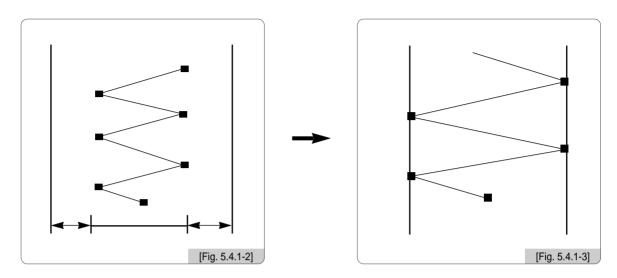
This function determines the satin stitch length in the X-axis direction. The value can be increased by the unit of 0.1mm.
