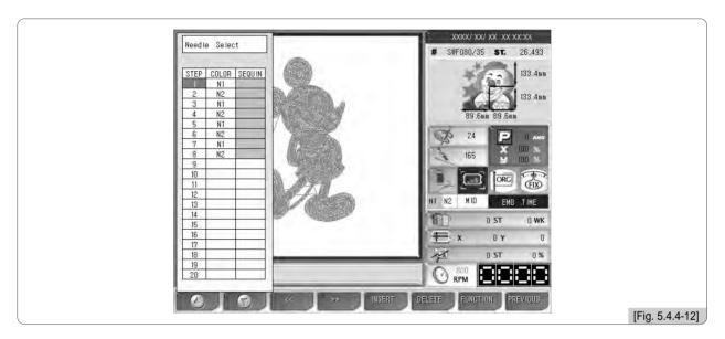
3 When F7 FUNCTION is pressed on the needle bar select screen as in <Fig. 5.4.4-12>, the screen appears as in <Fig. 5.4.4-13>. Press F5 CONVERT.
