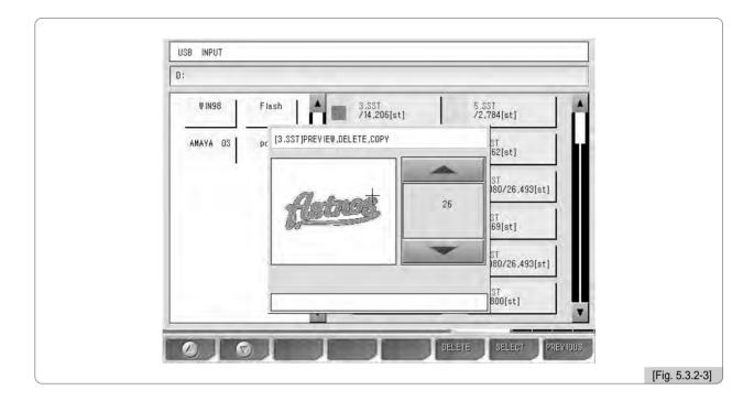
When a USB memory is used, the preview function is directly performed. Input and Delete function keys appear at the bottom. Preview, Delete, and Copy function can be used in the same way as in "5.3.1 FDD Input".
